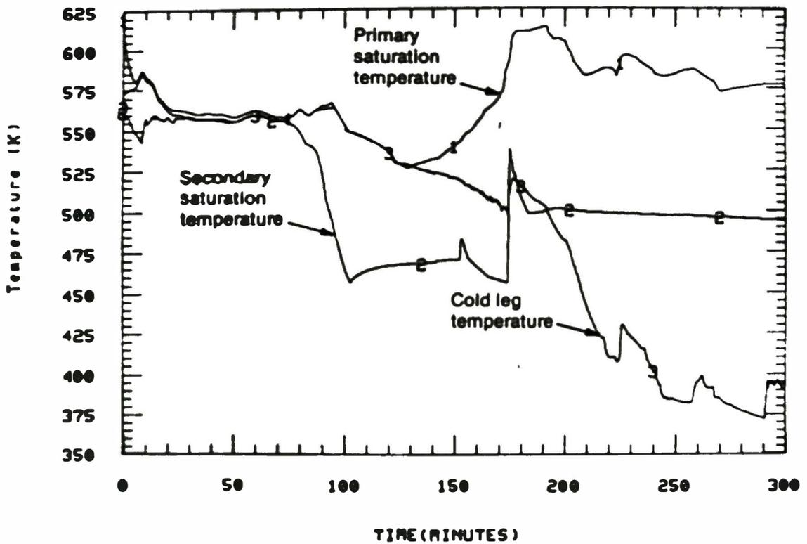
Figure 4. Comparison of primary saturation with B-loop secondary saturation and cold leg temperatures.
