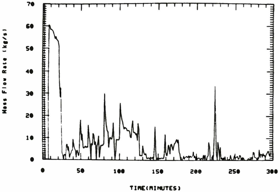
Figure 1. A-loop OTSG primary side condensation rate due to OTSG heat transfer.
