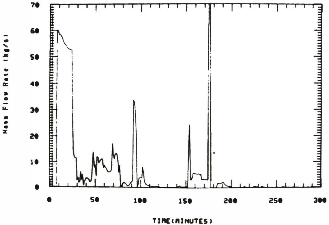
Figure 2. B-loop OTSG primary side condensation rate due to OTSG heat transfer.
