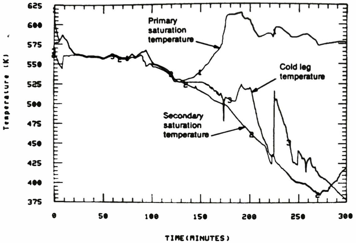
Figure 3. Comparison of primary saturation with A-loop secondary saturation and cold leg temperatures.
