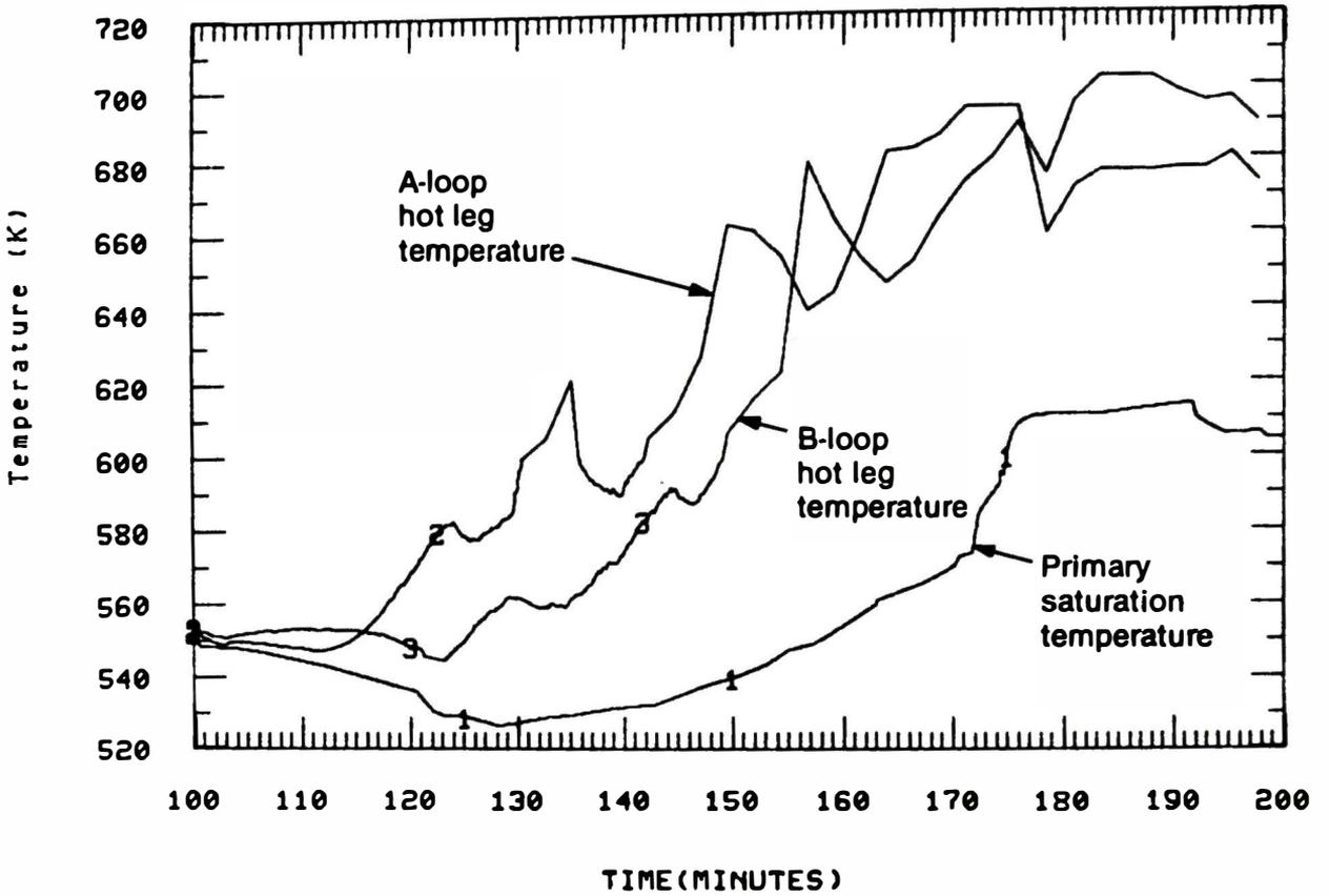
Figure 5. Comparison of primary saturation temperature with the measured hot leg temperatures.
